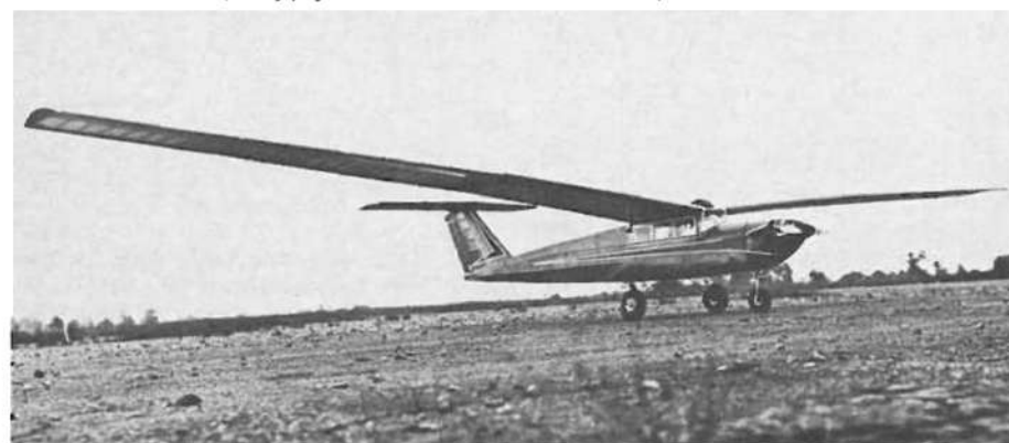
A T-tail configuration, high above the weeds and things. The polyhedral wing and the strip structure bring back remembrances of the 1950 decade. A huge, roomy fuselage for any experimental gear you might plan to try. It could mount cameras, carry payload. It flies well with the normal planform.
