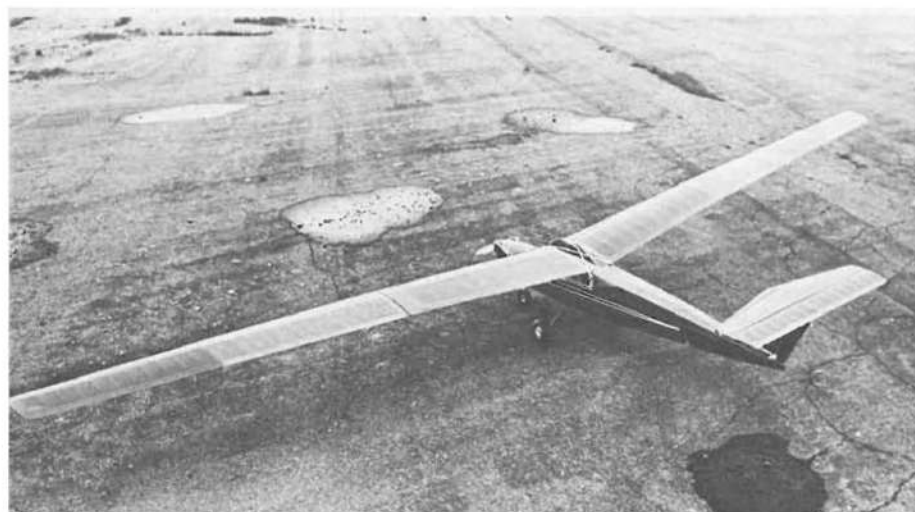
Kurwi wing panels attached to a tapered six-foot center-section. A drooped look on the ground, but it assumed polyhedral under flight loads imposed. The trike gear with a steerable coil spring commercial nose gear. Original utilized Tatone engine mount on a turned aluminum base.
