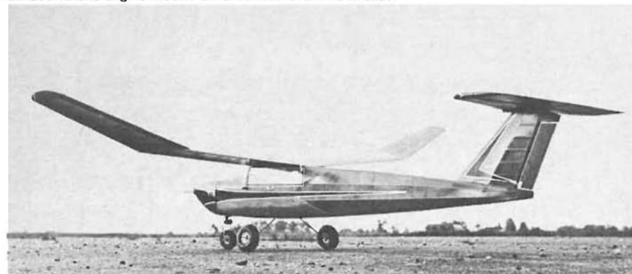
A T-tail configuration, high above the weeds and things. The polyhedral wing and the strip structure bring back remembrances of the 1950 decade. A huge, roomy fuselage for any experimental gear you might plan to try. It could mount cameras, carry payload. It flies well with the normal planform.
